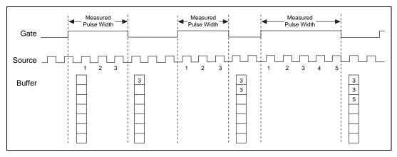
Figure 2-30. Buffered Pulse Width when Gate Is High during Arming
